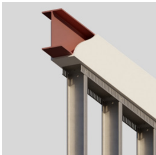
» Figure 1: Connection through encasement board
