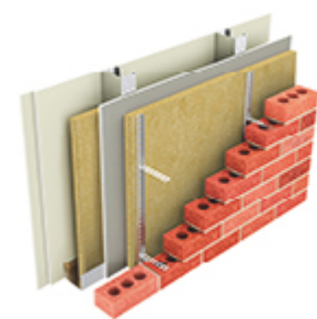
Option 1 Type EC1i: Two layers of minimum 12.5mm British Gypsum Fireline plasterboard, stud with ISOVER 50mm APR 1200 between, sheathing board, Rockwool Duo Slab Insulation, 50mm cavity, brickwork.
