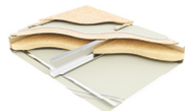
Option 5 Type F9: Three layers of 15mm British Gypsum Fireline plasterboard, Metsec RB565 resilient bars, joists with 1 x ISOVER 50mm APR 1200 quilt to cavity, 15mm plywood, 19mm British Gypsum Plank, 70mm Collecta Deckfon acoustic battens, 18mm V313 chipboard.
