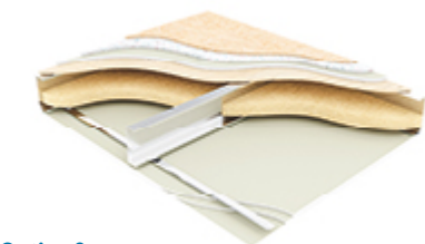
Option 2 Type F5: Three layers of British Gypsum Fireline plasterboard, Metsec RB565 resilient bars, joists with 1 x ISOVER 50mm APR 1200 quilt to cavity, 15mm plywood, 19mm British Gypsum Plank, 8mm Cloud 9 Underlay, 12mm OS
