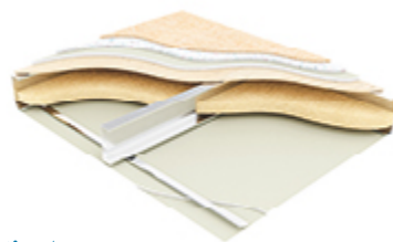
Option 4 Type F5: Three layers of 15mm British Gypsum Fireline plasterboard, Metsec RB565 resilient bars, joists with 1 x ISOVER 50mm APR 1200 quilt to cavity, 15mm plywood, 19mm British Gypsum Plank, 8mm Cloud 9 Underlay, 12mm OSB.
